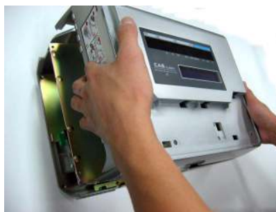
Open up from printer side to disassambel front cover
