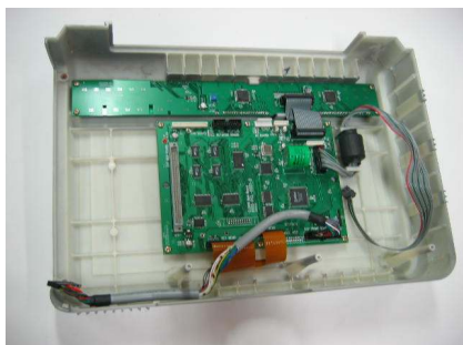
2. Remove support fram and replace main board.
