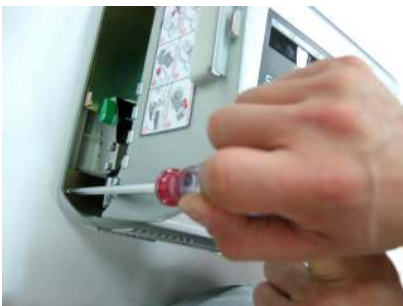
Remove front cover bolt (2 bolt)
