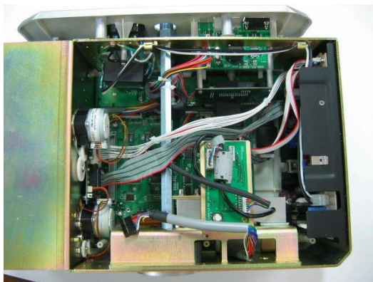
1. remove power cable from SMPS and ground wire.
