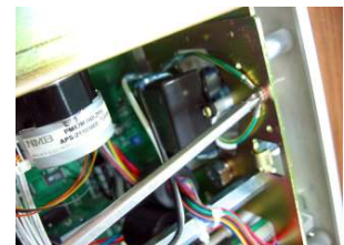
1. remove power cable from SMPS and ground wire.
